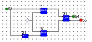
If 53 is set, the FlipFlop will also set (54:1). If 53 is reset, the FlipFlop will also reset (54:0).
